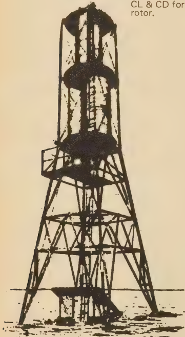
VERTICAL-AXIS DOUBLE SAVONIUS WINDMILL-TYPE F-13 OF THE SOVIET WIND ENERGY INSTITUTE
